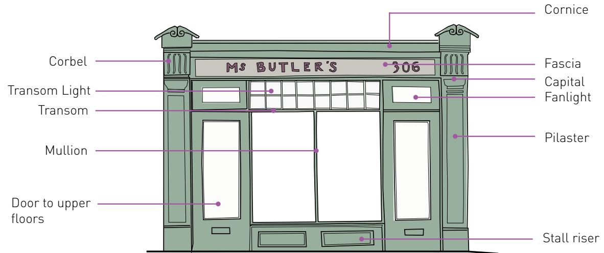
One example of a traditional shopfront layout
