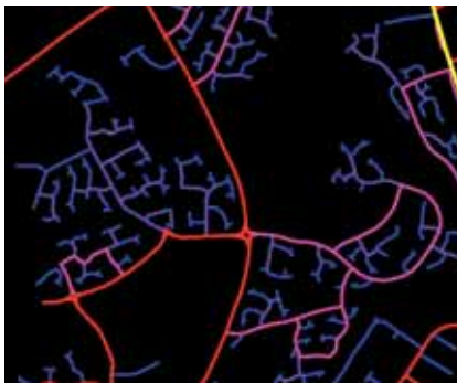
Loops and cul-de-sacs (in magenta, violet and blue) create longer routes for many journeys making walking less attractive
